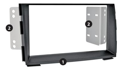
(1) Double DIN Facia Plate(2) Mounting brackets (left/right)
