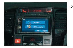
5. Attach brackets to Double DIN head unit. Connect all required circuit points. Fix Double DIN double DIN head unit at dashboard. Place facia plate until it snaps in. Reinstall everything in reverse order to finish installation
